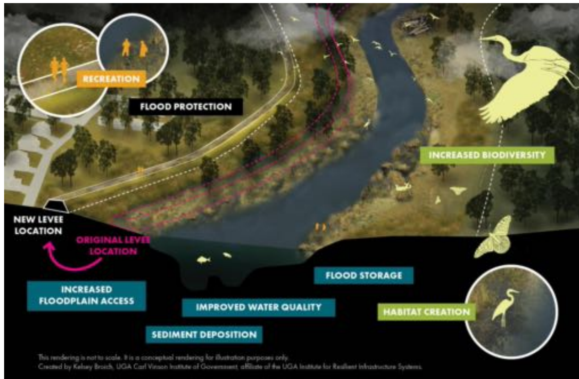
Figure 2. A graphic of a levee setback, which reconnects a river to its historic floodplain.
